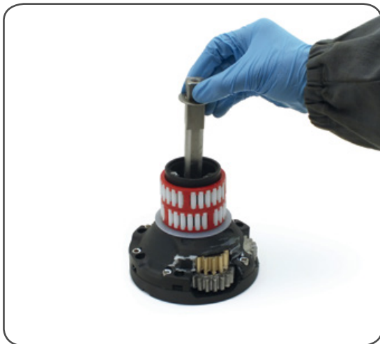
6. Slide out the central shaft n°18
