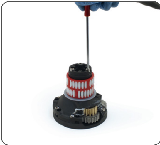
4. Completely unscrew the three screws n° 28
