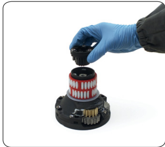
5. Remove the socket support n°20
