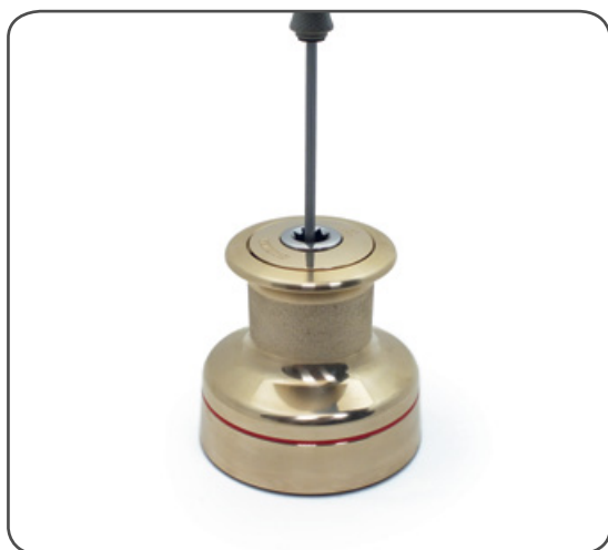
1. Unscrew the central screw ( \approx 2\text{Nm}/18\text{ in-lb} )
