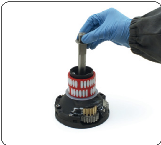
6. Slide out the central shaft n°18
