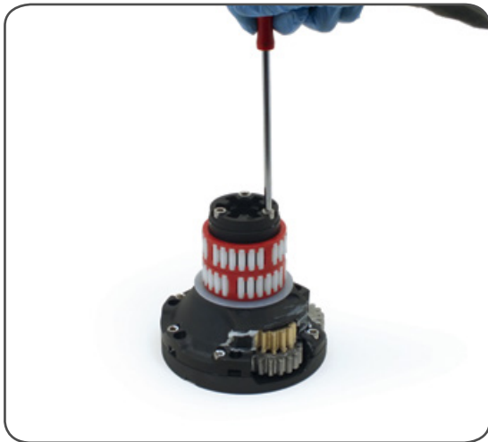
4. Completely unscrew the three screws n° 26
