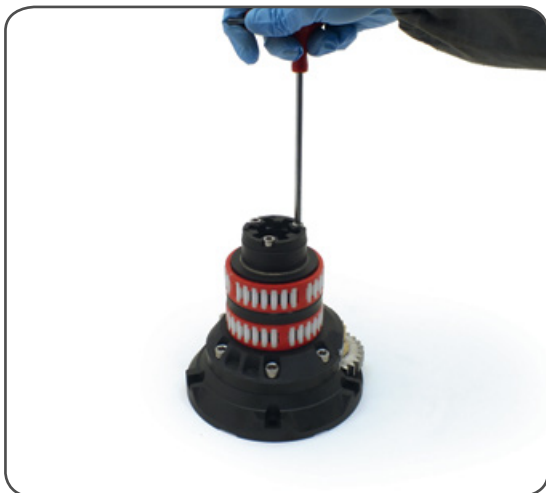
4. Completely unscrew the three screws n° 27
