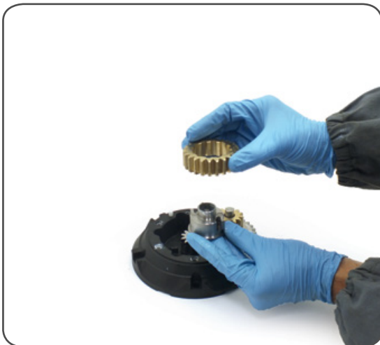
To facilitate the operation press the spring against the pawl with a blade.
