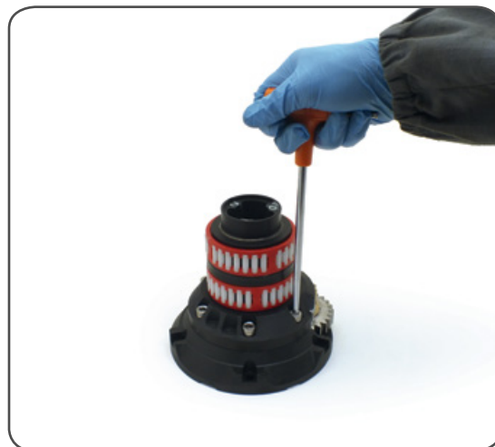
7. Unscrew the 5 hex screws n°16 ( \approx 8\text{Nm}/71\text{ in-lb} )
