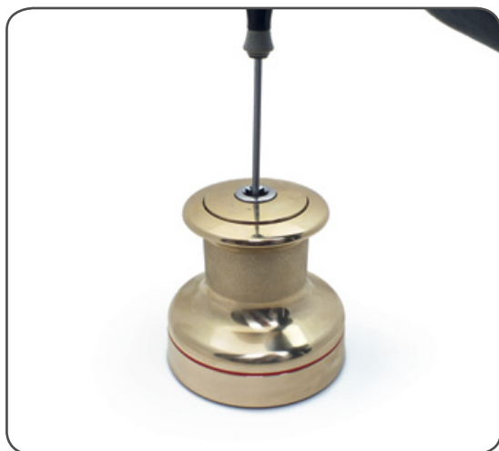
1. Unscrew the central screw ( \approx 2\text{Nm}/18\text{ in-lb} )
