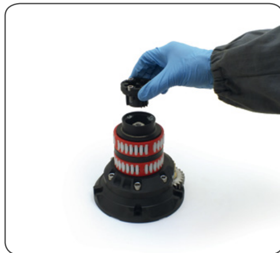
5. Remove the socket support n°21
