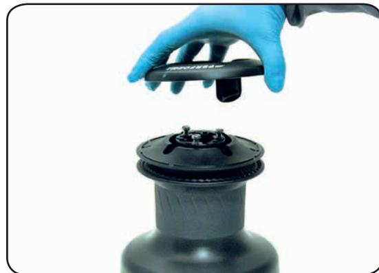
4. Remove the stripper arm n°26 by rotating and lifting it.
