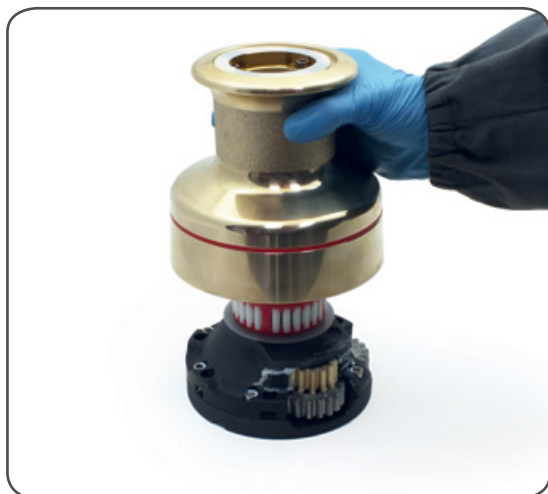
3. Lift off the drum n°23
