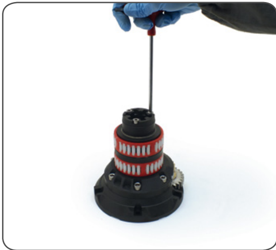
4. Completely unscrew the three screws n° 28
