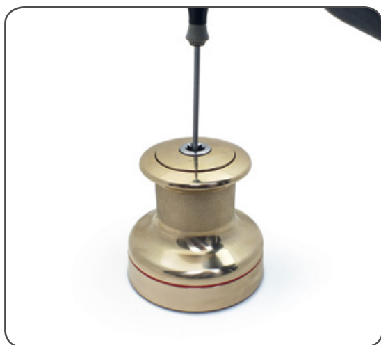
1. Unscrew the central screw ( \approx 2\text{Nm}/18\text{ in-lb} )
