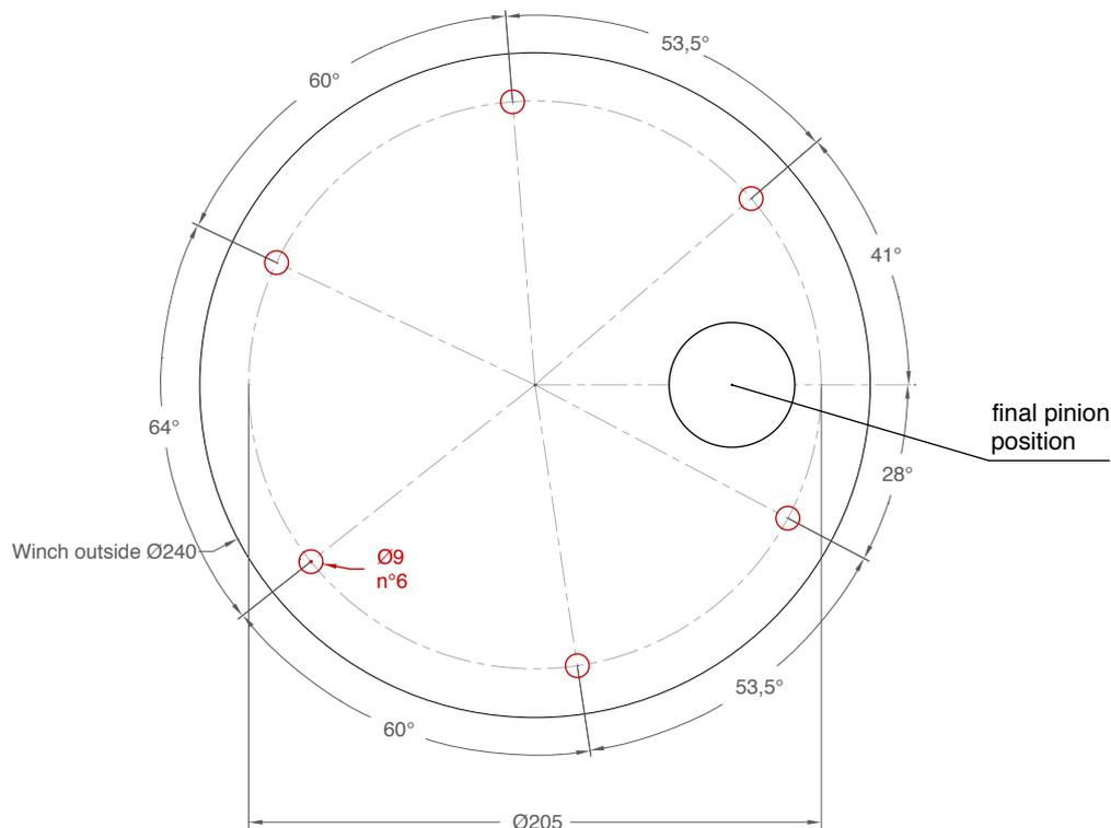
**B.** Remove the winch and drill the six 9 mm diameter holes.
