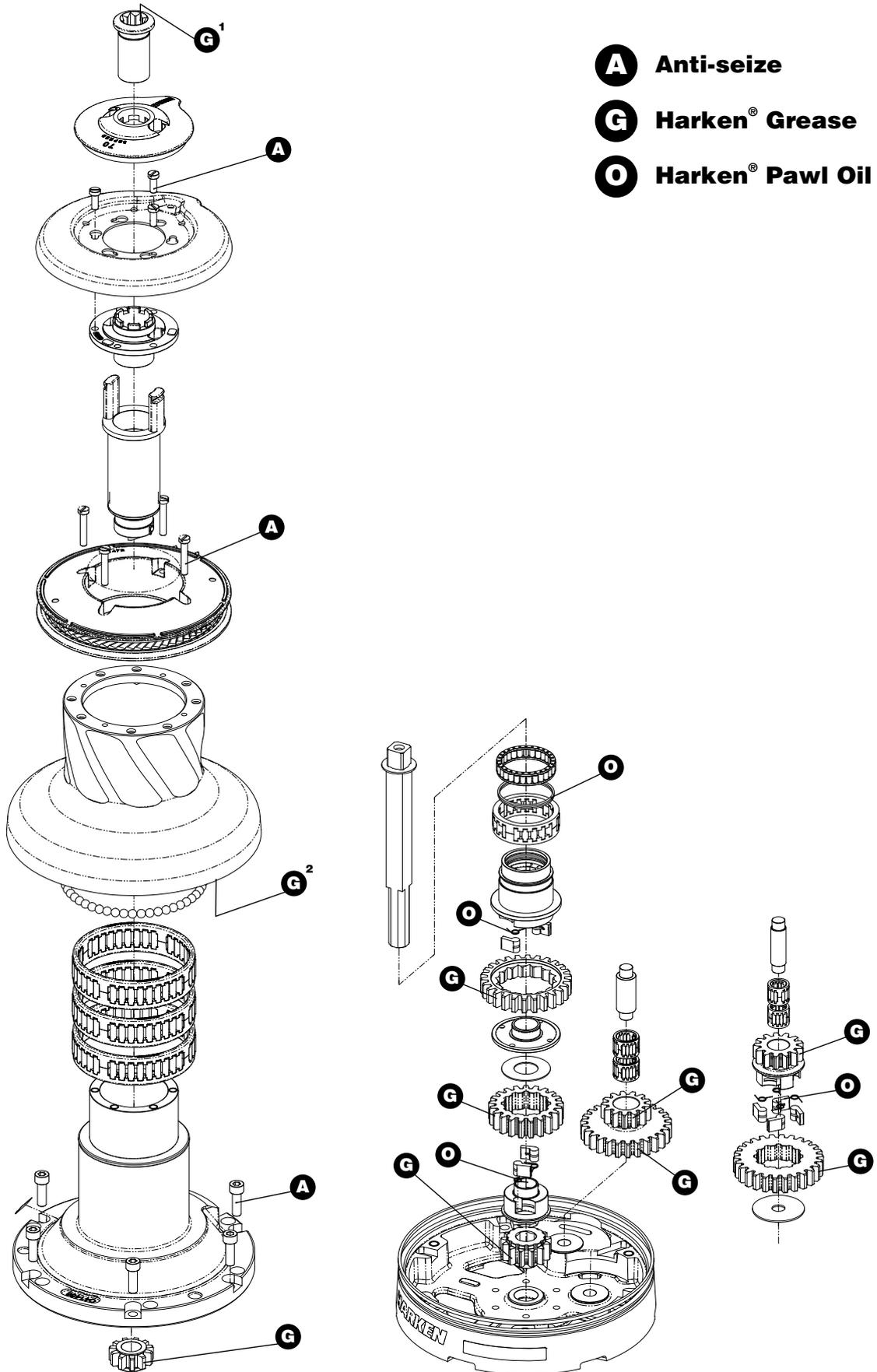
1. Apply Harken® grease on assy socket screw - 2. Apply Harken® grease on drum gear
