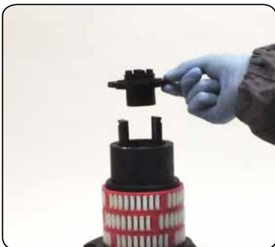
6. Remove the stripper arm housing n°21
