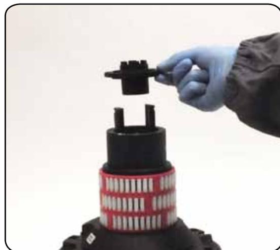
6. Remove the stripper arm housing n°21
